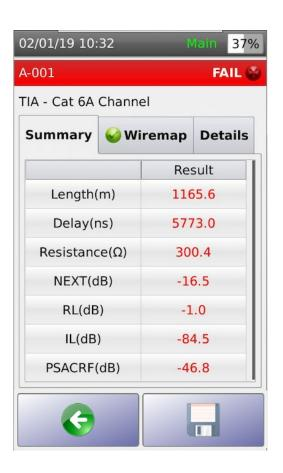
Note: Tests will fail using Standards-based test limits such as Cat6A channel, as longer cables will not pass due to the limits set by the standards. TestPro allows importation of custom limits to accommodate long cables.
