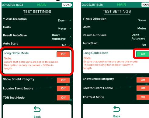
3. **Important!** Repeat steps 1 and 2 above for the TestPro Remote unit. Both Main and Remote must be set to Long Cable mode.
