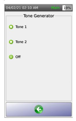
The tones are generated on all 8 conductors to ensure good cable location function regardless of possible wire map issues.
