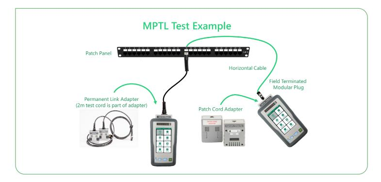
13. MPTL or Modular Plug Terminated Links almost consists of a permanent link consisting of wall-mount jacks at one end of cabling and patch panel at the other end and Patch-cords to connect networking end-points to wall-mount jacks at both ends, wherein the entire cabling including the patch-cords (but not the plugs at the end-point connections) is referred to as the channel.
