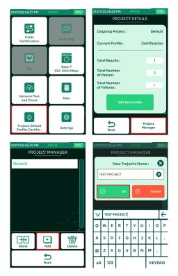
b. When prompted, hit yes to set your project as the current project, then select the profile type "Copper Certification" and click save in lower right corner. Hit the "Back" button and current Project (name) and Profile (Certification) at the top.
