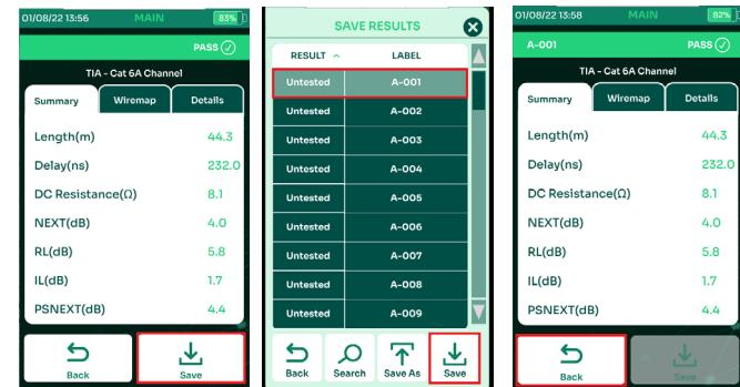
11. After test is saved, hit Back button. Continue to the next cable to be tested and repeat Steps 9 & 10.
