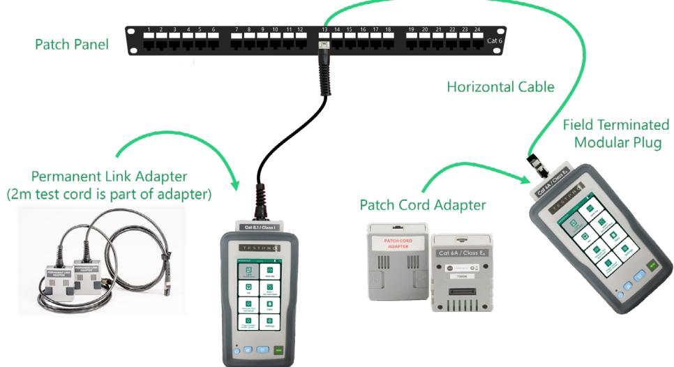
13. MPTL or Modular Plug Terminated Links almost consists of a permanent link consisting of wall-mount jacks at one end of cabling and patch panel at the other end and Patch-cords to connect networking end-points to wall-mount jacks at both ends, wherein the entire cabling including the patch-cords (but not the plugs at the end-point connections) is referred to as the channel.
